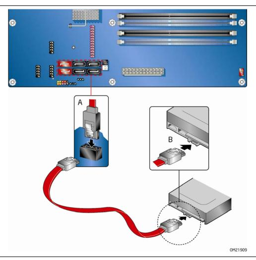
Figure 19. Connecting a Serial ATA Cable
